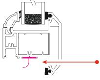
Fit a Sash Spring to the sash on the center line of the stay fixing area
